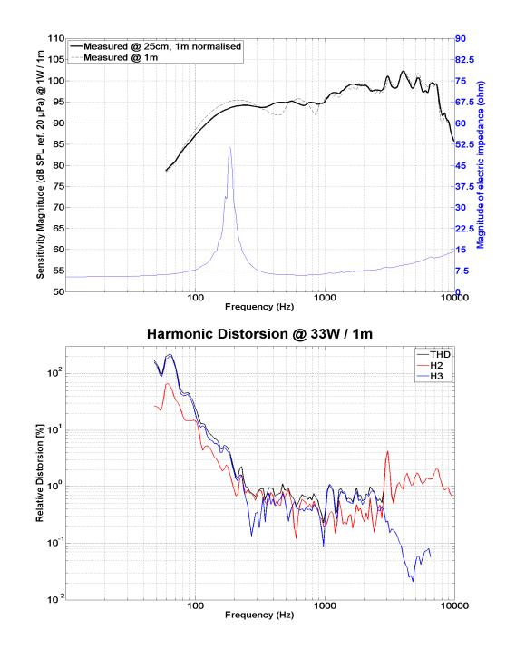
HD curve measured on CEI standard baffle : . at 1 meter . at power = P\_AES / 4
