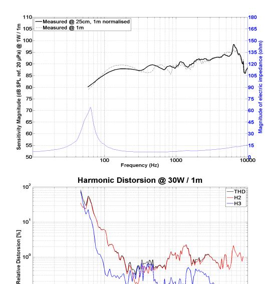
HD curve measured on CEI standard baffle :
